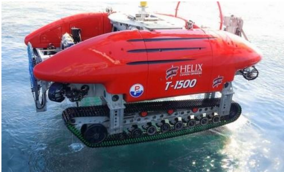
Figure 6-5 : Example Jet Trencher (Helix T1500)
