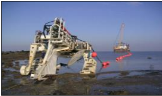
Figure 6-3 : Hi-plough, pull to offshore
